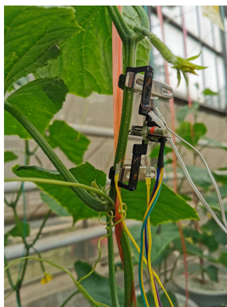
Figure 11. Schematic diagram of sensor installation.
