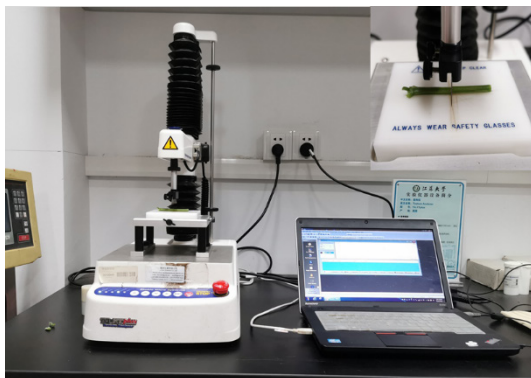
Figure A2. Shear test of stem on the 7th day of installation.
