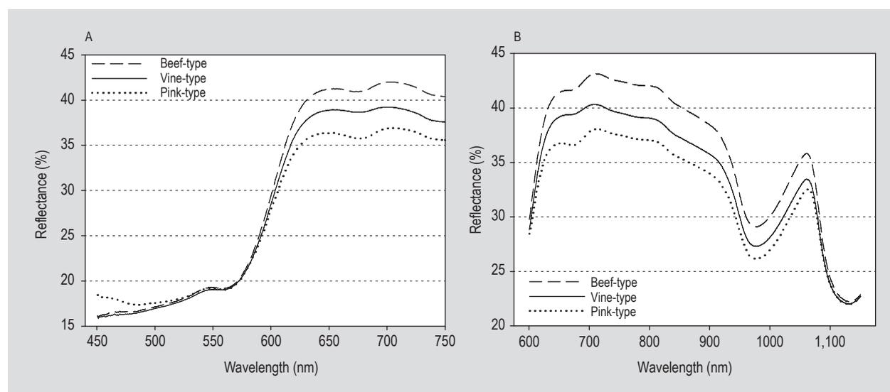
**Figure 1. Average reflectance profiles obtained from the (A) visible spectrometer and (B) visible-near-infrared spectrometer.**
