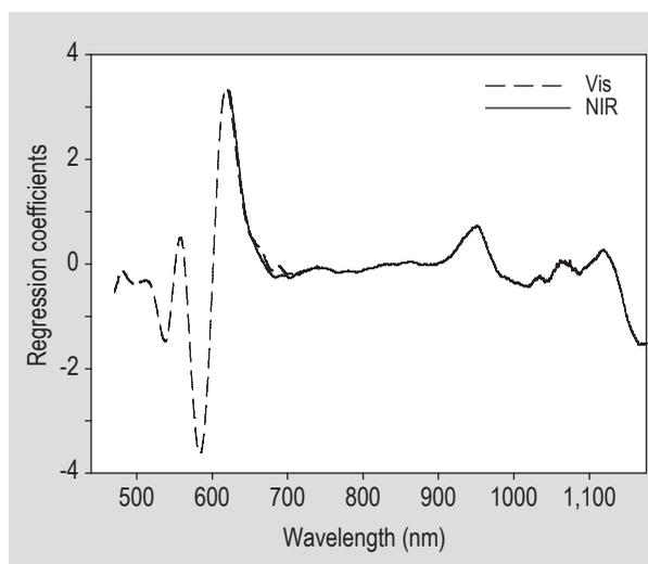
**Figure 3. Regression coefficients of partial least squares-models for spectral analysis of lycopene content obtained from combined visible (Vis; 450-750 nm) and near-infrared (NIR; 600-1,150 nm) spectrometers with 3 latent variables. Models based on mean normalised spectra including all three tomato fruit types.**
