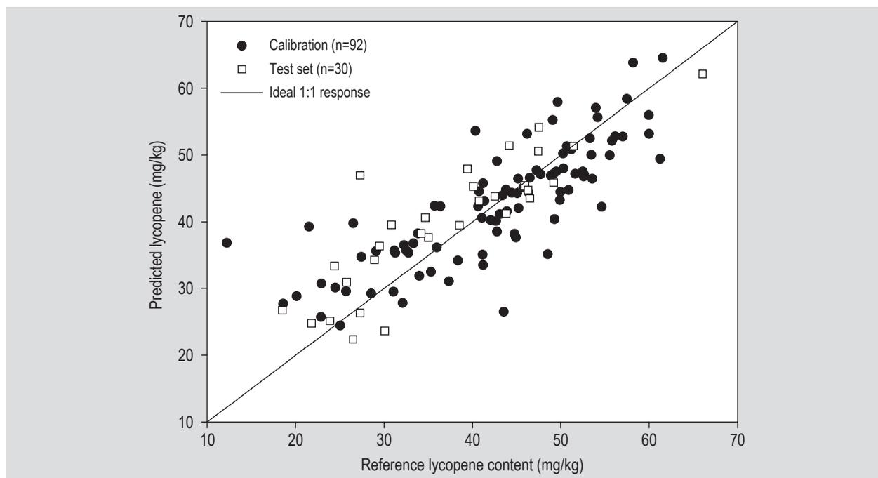
**Figure 2. Prediction of lycopene content of beef-type fruits by visible + near-infrared spectroscopy using a solid-state device. Validation test set results:  $r^2=0.75$ , RMSEP=6.07 mg/kg.**
